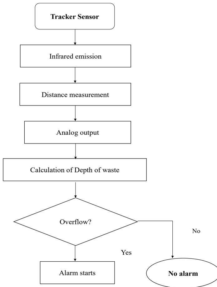
Figure 3. Flowchart of the ESS-IoT system algorithm for waste collection
